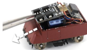
The contact points for the decoder are thus exposed. You can now plug in the decoder. Pay attention to the correct installation position. Information on this can be found in the instructions for the decoder. When installing the housing later, make sure that it is in the correct position and that no cables etc. are pinched.
